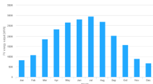
Monthly energy output from fix-angle PV system:
